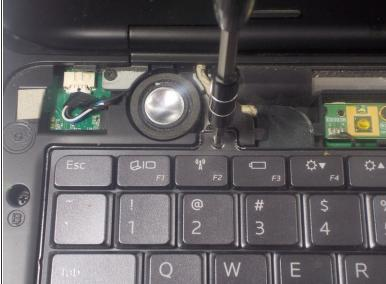
• Use a JIS 1 screwdriver to remove (2) 2.5mm screws located near the top of the keyboard.
