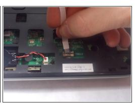
Disconnect the track pad cable by flipping up the gray clamp and lifting the cable up.
