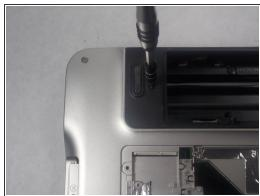
Use a JIS 1 screwdriver to remove (2) 7mm screws on the underside of the laptop near the battery bay.
