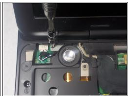
Remove (2) 4mm screws with a JIS 1 screwdriver that are holding down the left side display anchor.
