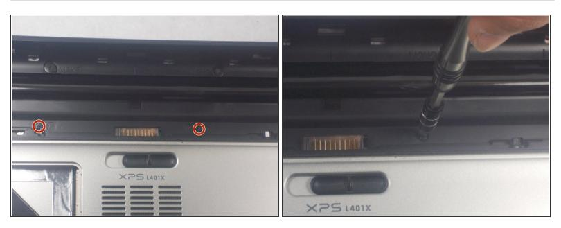
Remove (2) 4.5mm screws with JIS 1 screwdriver marked by the letter "K" near Battery
