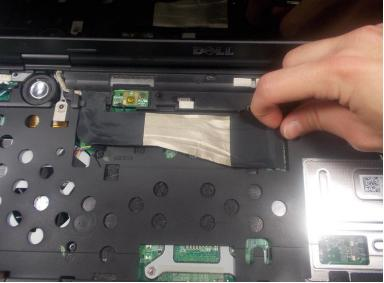
Disconnect the display ribbon cable by pulling the cable to the right by its sheathed plastic connector.
