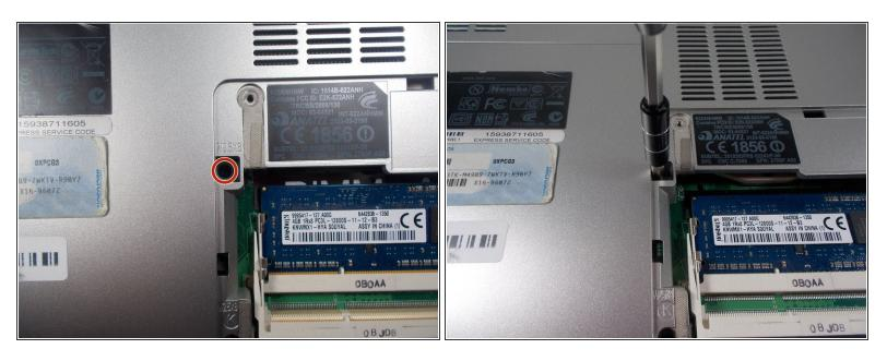
Locate and remove (1) 8.5mm JIS 1 screw at the top left corner of the RAM bay.
