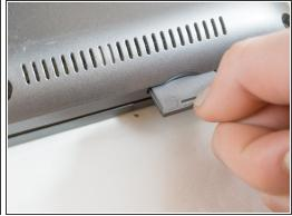
• Using your fingers, pinch the edge of the SD card and pull to remove it.
