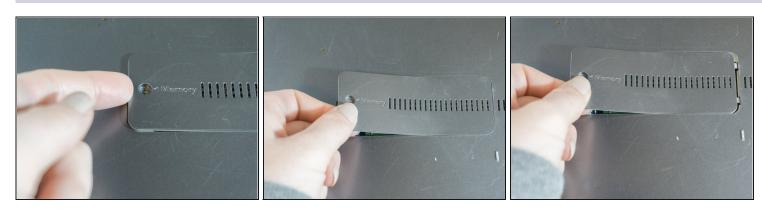
• Wedge your finger underneath the edge of the memory cover. Grasp and pull the cover to the left to remove it.
