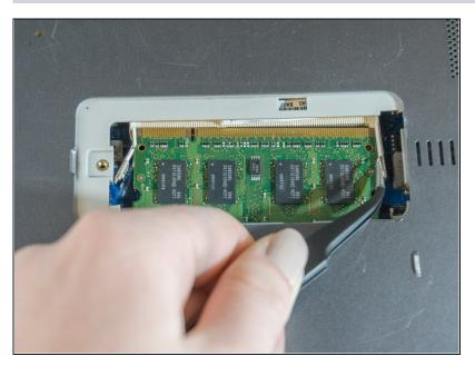
Using the tweezers, push the edges of the metal clasps holding the ram card away from the card. You should see the card pop upwards.
