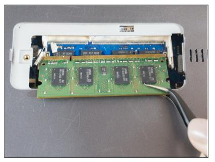
Using the tweezers, grasp the ram card and pull straight out to remove it.
