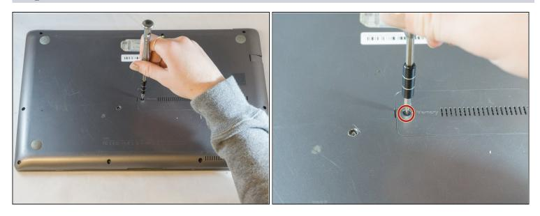
• Using the Phillips #00 screwdriver, remove the 6.6mm screw from the memory slot cover.
