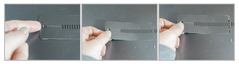
• Wedge your finger underneath the edge of the memory cover. Grasp and pull the cover to the left to remove it.
