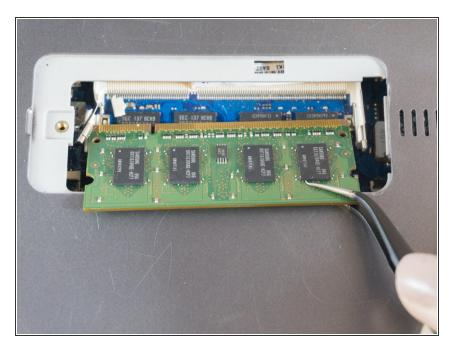
Using the tweezers, grasp the ram card and pull straight out to remove it.
