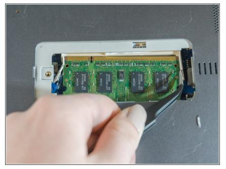
Using the tweezers, push the edges of the metal clasps holding the ram card away from the card. You should see the card pop upwards.
