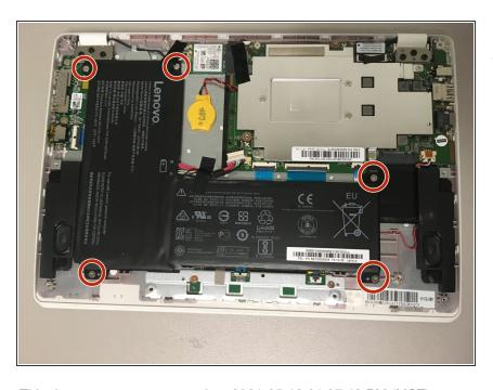
Remove the five 4 mm Phillips screws securing the battery.
