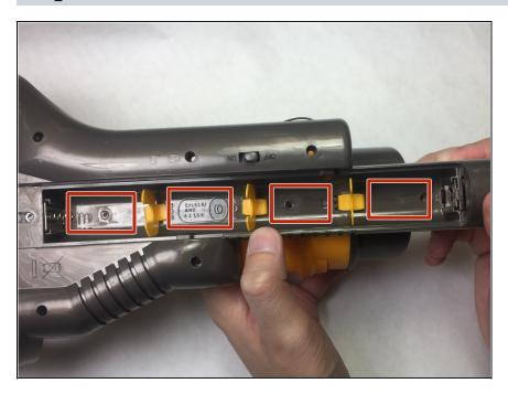
Remove batteries from the vacuum by pulling them out and away from the vacuum.
