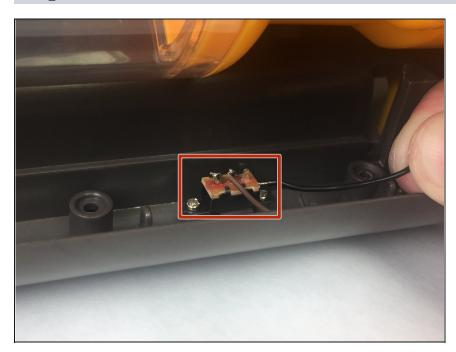
Cut the two wires connected to the on/off switch using a set of wire cutters.
