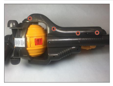
Remove four 9.2mm (0.32 in) screws from the back of the vacuum using the PH00 screwdriver.
