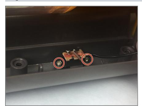
Remove the two 9.2mm (0.32 in) screws which hold the on/off switch to the vacuum using the PH00 screwdriver.
