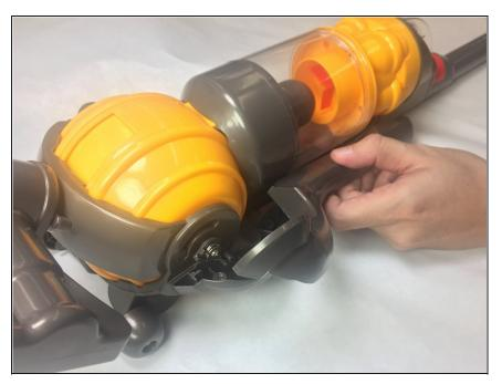
Remove the cover to the on/off switch by pulling up on the cover from the front of the vacuum.
