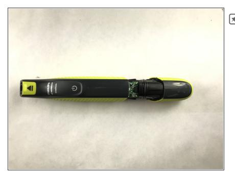
Power button should face forward in same direction as circuit board. The crease on each casing component should line up.
