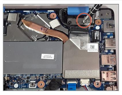
Unscrew the four screws with a Phillips screwdriver.
