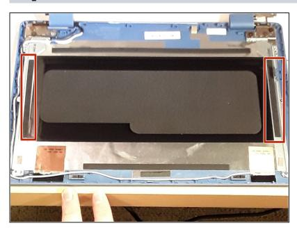
Locate the metal hinge on each side of the blue half of the screen.
