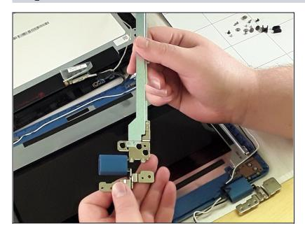
• Pull off the blue plastic located at the top of the hinge.
