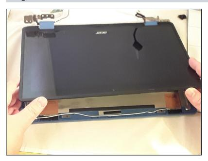
• Insert the tip of the metal spudger at the seam to pry the screen display from the cover.
