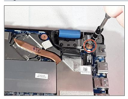
Remove the four 12.7 mm PH#0 screws that are surrounded by a copper ring.
