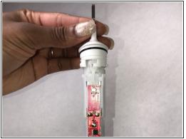
Using the pliers, rotate the head base 90 degrees counterclockwise and remove core from the handle.
