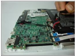
Carefully disconnect the battery cable from its connector on the mainboard.
