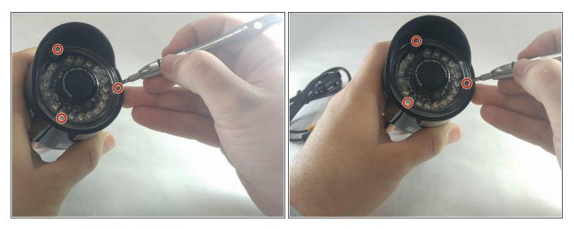
To remove the circuit board, you must begin by removing the three screw caps and the 15mm JIS
