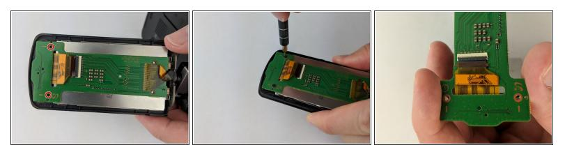
Locate and remove the two 3.5mm Phillips #00 screws holding the back cover.
