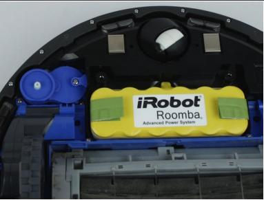
Remove the 4 screws holding the main bottom plate on and pull the plate away from the body.
