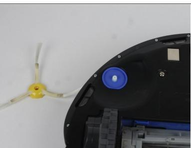
Flip over the Roomba and remove the side brush using a PH2 screwdriver.
