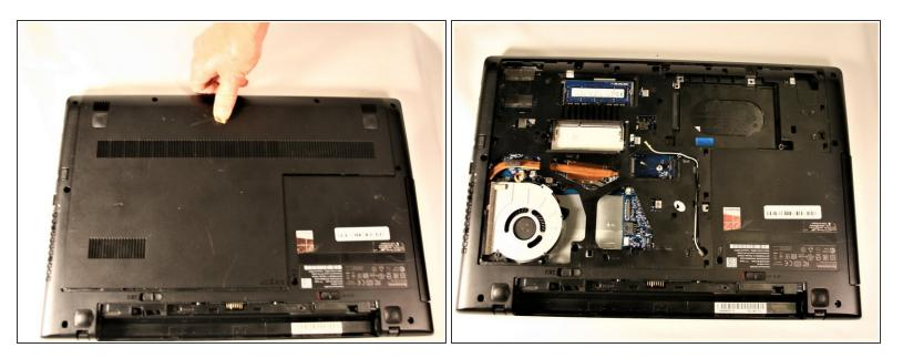
• Slide the cover away from the hinges and lift the panel off.
