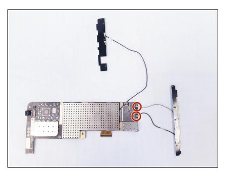
Disconnect the antenna module from the motherboard. To reassemble your device, follow these instructions in reverse order.
