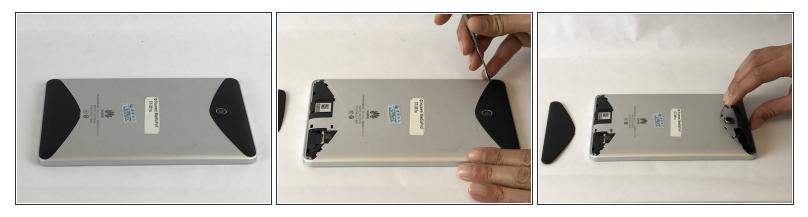
• Use either your finger or a metal spudger to lift both the top and bottom black covers on the back of the tablet.
