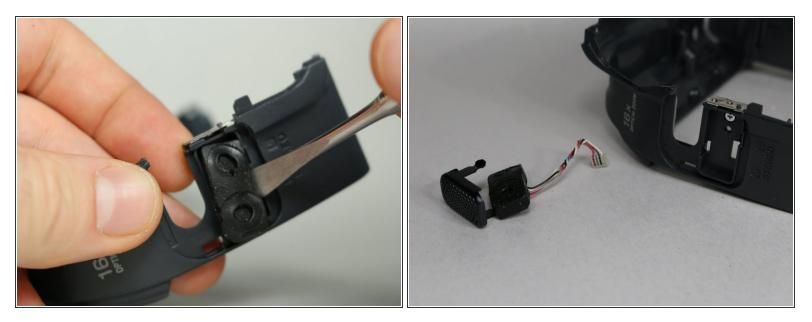
• Use a metal spudger to lift the microphone out of its housing.
