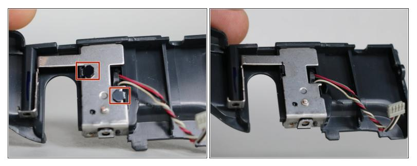
Pry up the two tabs and push them to remove the microphone cover.
