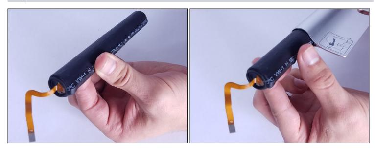
• Replace the old battery with the new battery
