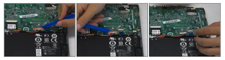
• Dislodge the battery's connector to the motherboard by using the plastic opening tool as a lever on the two small plastic tabs that stick out on either side of the connector.
