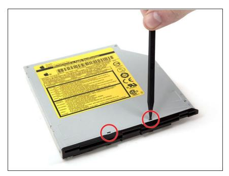
Use a spudger to depress and release the two black tabs on top of the optical drive directly over the bezel.
