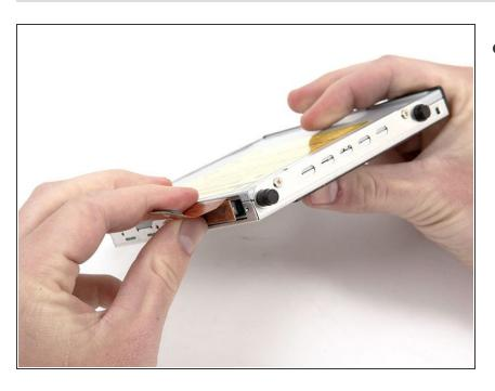
Disconnect the orange optical drive ribbon from the back of the drive.
