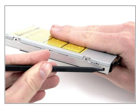
Use a spudger to depress and release the black tab on the left side of the optical drive.
