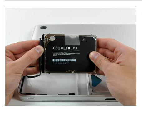
Remove the hard drive from its cable by pulling the cable connector straight away from the drive.
