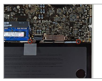
Remove the two 7.4 mm Tri-point screws securing the battery to the upper case.
