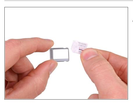
Remove the SIM card from its recess in the SIM card tray.
