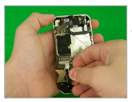
Using your fingers or a plastic opening tool carefully pull out the logic board.
