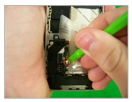
• Disconnect the antenna cable from the logic board.
