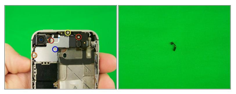
• Unscrew the 4 screws holding the large shield and the single screw holding the small shield.
