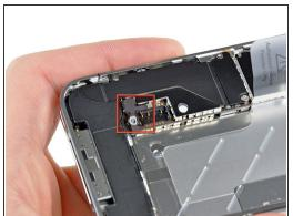
Use an iPod opening tool to carefully pry the battery connector up from the ends closest to the top and bottom edges of the iPhone.
