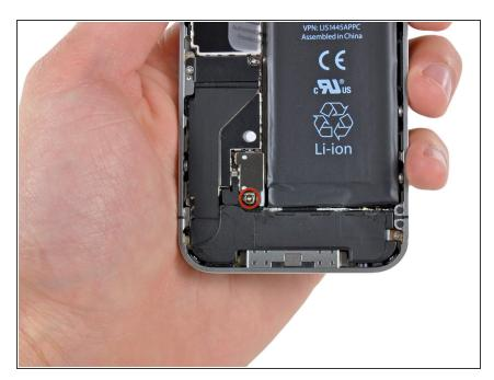
Remove the single 2.5 mm Phillips screw securing the battery connector to the logic board.
