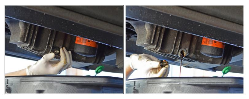
Remove the oil drain plug and let any oil that has collected drain out.
