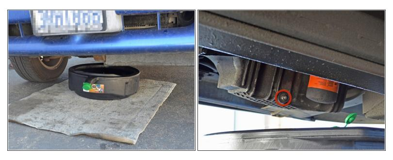
Slide an oil drain pan under the car in a position that oil from the oil drain plug (marked in red) will flow into it.
