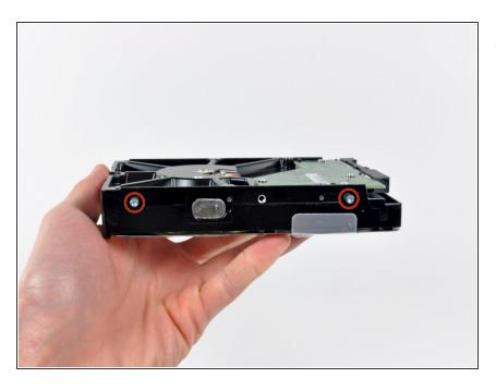
Remove the two T8 Torx pins from the other side of the hard drive.
