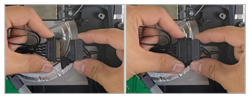
• Connect the iMac's SATA power cable to the other end of the new sensor-enabled SATA cable.
