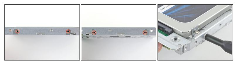
• Use a Phillips screwdriver to install the four silver screws (two on each side) along the edges of the SSD to secure it to the enclosure.
