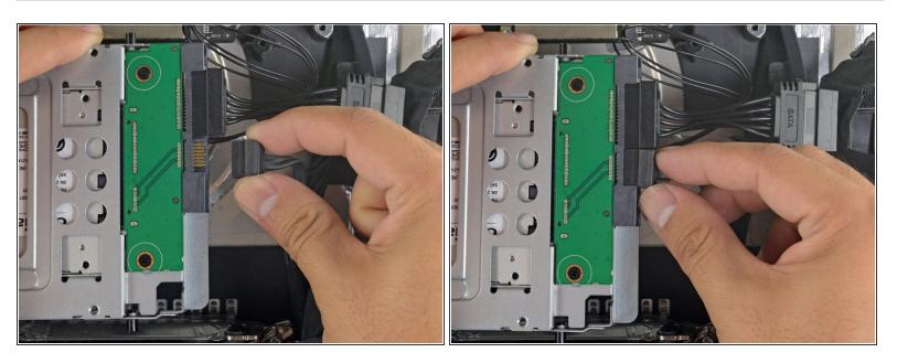
Connect the iMac's SATA data cable to the enclosure's socket.
