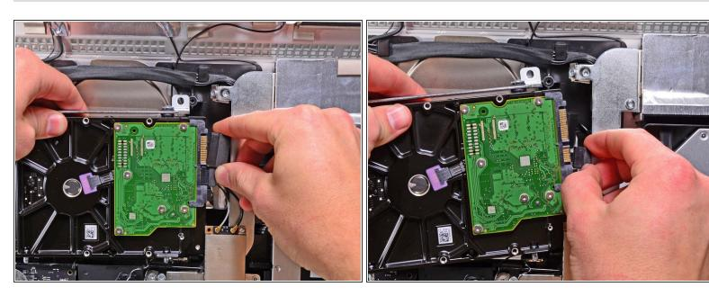
Disconnect the SATA data cable and SATA power connector from their respective sockets by pulling each connector away from the hard drive.
