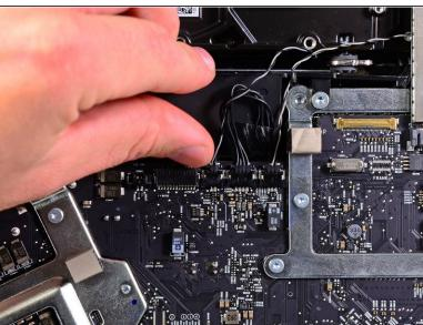
Pull the hard drive temperature sensor connector toward the top edge of the iMac to disconnect it from its socket on the logic board.
