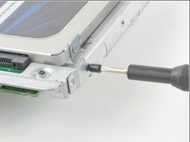
Use a T8 driver to install the mounting pins from the old hard drive onto the sides of the enclosure.
