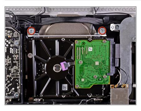
Remove the two 9 mm T10 Torx screws securing the upper hard drive bracket to the outer case.
