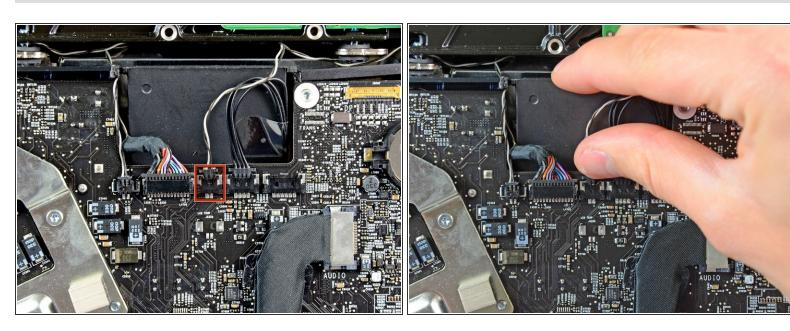
Pull the optical drive thermal sensor connector straight up from its socket on the logic board. Pull parallel to the board.
