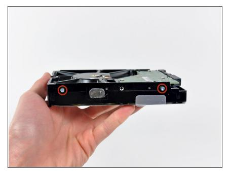
• Remove the two T8 Torx pins from the other side of the hard drive.
