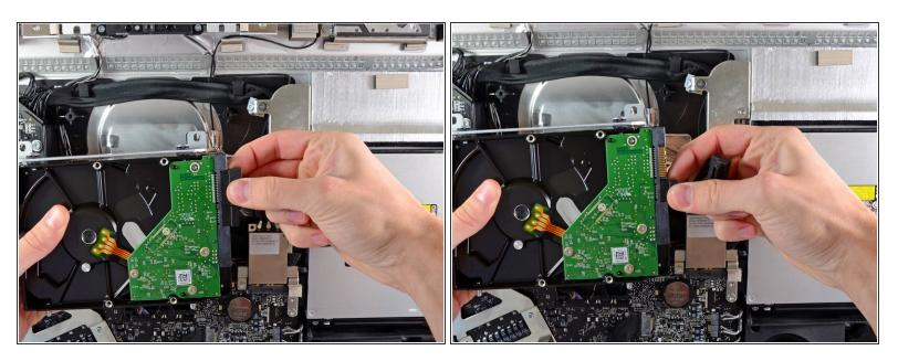
Disconnect the SATA data cable and SATA power connector from their respective sockets by pulling each connector away from the hard drive.
