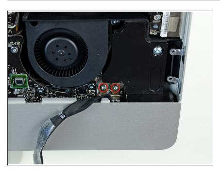
Remove two 5 mm T10 Torx screws securing the audio ports to the outer case.
