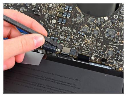
• Use the flat end of a spudger to pry the trackpad connector up and out of its socket on the logic board.
