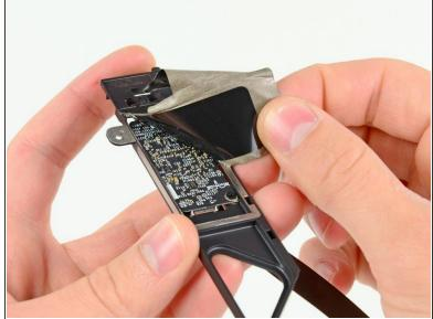
Peel and remove the piece of EMI tape wrapped around the AirPort/Bluetooth assembly.
