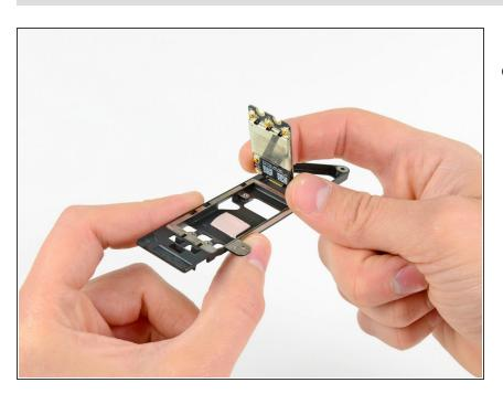
Remove the AirPort/Bluetooth board from its aluminum housing.
