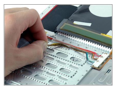
Peel up the Bluetooth data cable from the adhesive on the upper case.
