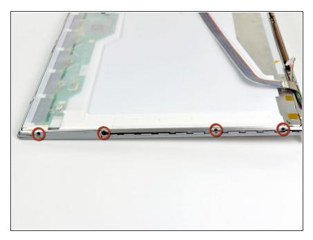
Remove the four 3.3 mm Phillips screws securing the right side of the LCD to the front display bezel.
