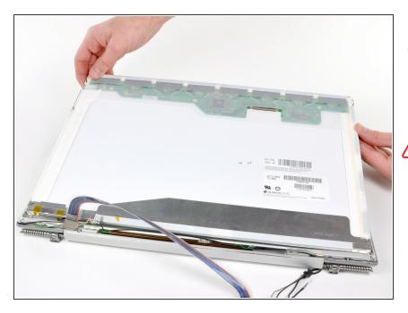
Lift the top edge of the LCD out of the front display bezel and slightly pull its bottom edge away from the clutch hinges.
