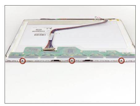
Remove the three 3.3 mm Phillips screws along the top edge of the LCD.
