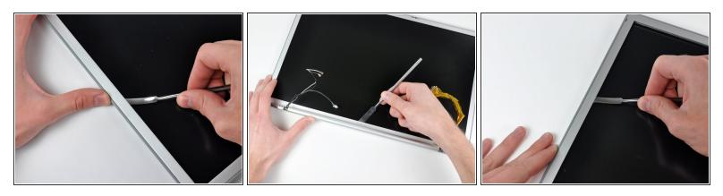
• Continue running the edge of your metal spudger between the LCD frame and the front bezel until the right, bottom, and left sides of the LCD are free.
