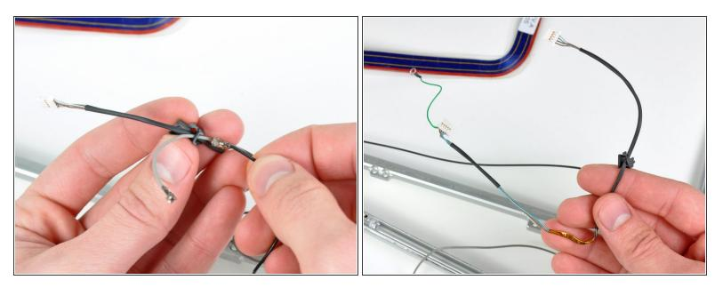
De-route both the black and the gray antenna cables through the black plastic cable retainer attached to the inverter cable.
