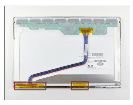
(i) If present, remove the pieces of tape stuck to the lower edge of the LCD.
