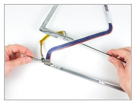
Remove the clutch hinges (with the display data cable still attached) from the front display bezel.
