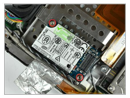
Use a 4 mm nut driver to remove the two nuts securing the modem to the PC card cage.
