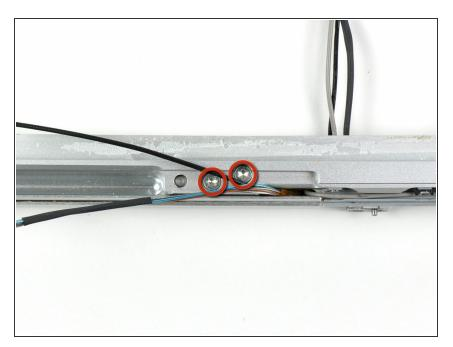
Remove the final pair of 10.3 mm T8 Torx screws securing the clutch hinges to the front display bezel.
