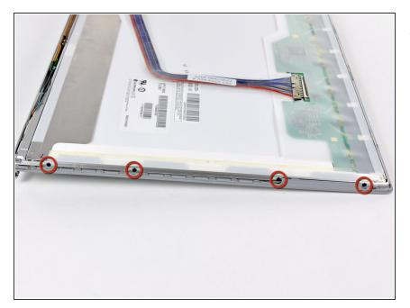
Remove the four 3.3 mm Phillips screws along the left side of the LCD.
