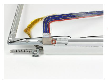
Remove the 2.7 mm Phillips screw securing the display data cable ground loop to the front display bezel.
