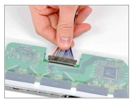
• Disconnect the display data cable from its socket on the LCD.
