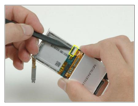
Use a spudger to flip up the black plastic tab holding the orange display ribbon in place. The tab will rotate up 90 degrees, releasing the ribbon cable.
