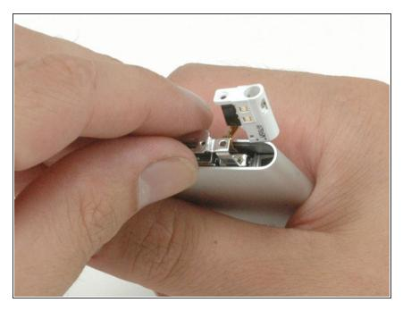
Lift the bottom bezel bracket out of the iPod.
