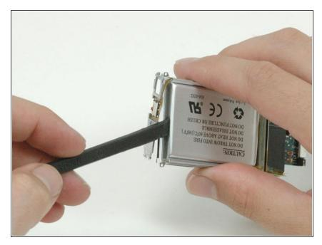
Use a spudger to gently pry the battery up from the back of the display. Be careful not to put too much pressure on the display with your spudger.
