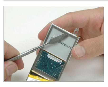
Use a metal spudger to carefully pry the metal bracket off the back of the display. Make sure you only pry off the bracket and not the clear shielding on the rear of the display. By working from the inside of the display, you won't be able to accidentially pry up the clear plastic shielding.
