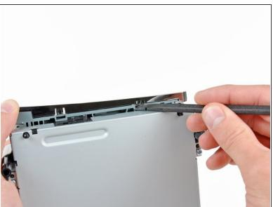
While pressing the optical drive cover toward the top face of the optical drive, use the flat end of a spudger to release the two retaining clips on the underside of the cover.
