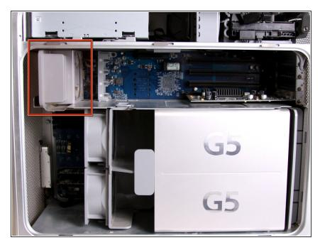
Locate the top left cooling fan unit.
