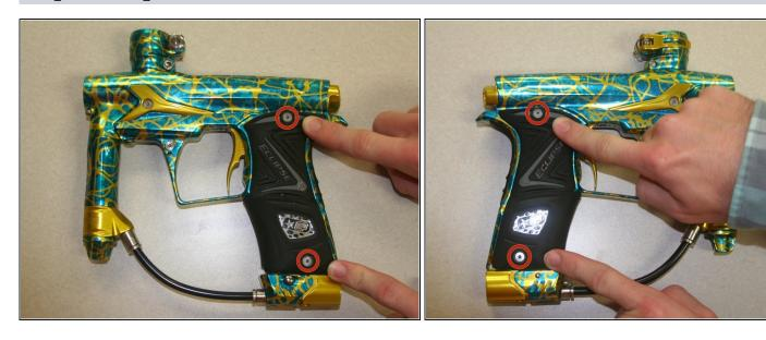
• Remove the four screws from the grip with the 5/64" allen wrench. There are two on each side.
