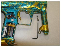
Use 1/8" allen wrench to remove screw behind regulator.
