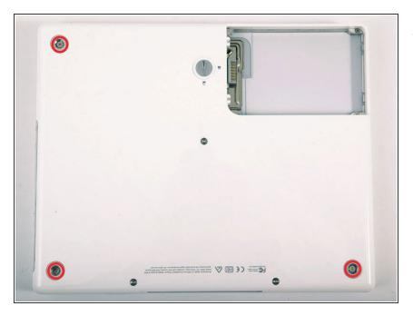
Remove the three newly-revealed Phillips screws.
