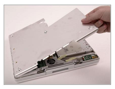
Lift the bottom shield off.
