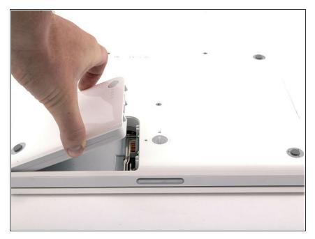
Lift the battery out of the computer.
