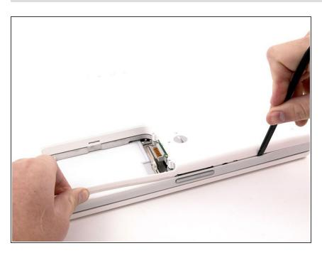
Run a spudger along the seam between the lower case and upper case on the front of the computer to free the tabs locking the lower case.
