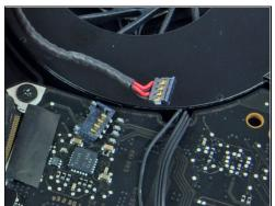
• Use the flat end of a spudger to pry the subwoofer/right speaker cable connector up off its socket on the logic board.
