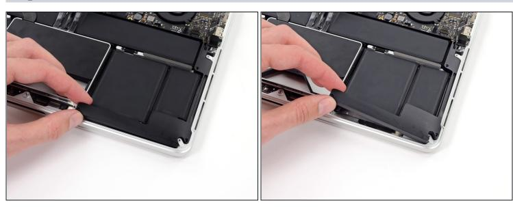
Lift and remove the left speaker out of the upper case.
