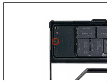
Remove the single 2.9 mm T5 Torx screw securing the SSD to the SSD tray.
