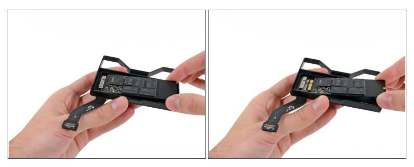
• Carefully pull the SSD straight out of its socket on the SSD tray.
