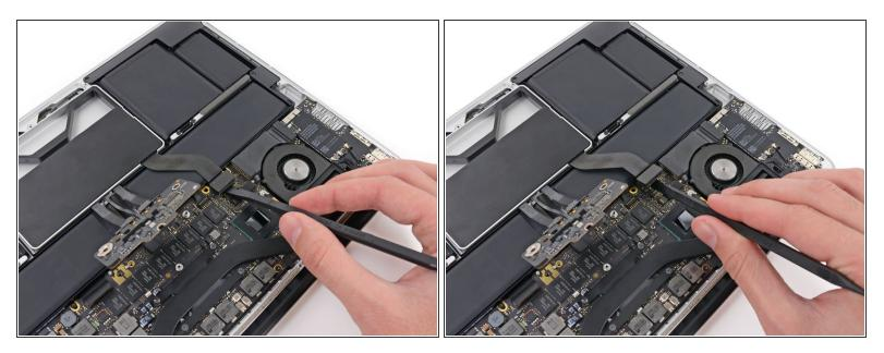
• Use the flat end of a spudger to pry the SSD cable connector up from its socket on the logic board.
